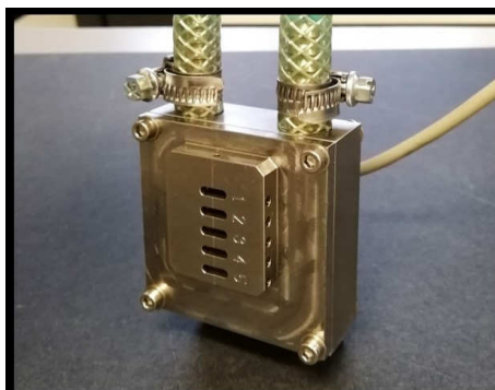
FIGURE 3.2: GALAXI sample holder for five capillaries. Inlet and outlet allow the circulation of water in the back of the holder in order to control the temperature of the samples.
